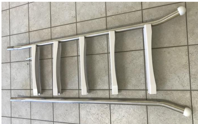
Use an 'opposite hand' leg. Top bend up. Foot points outwards. Step angle to suit the lean of the leg.
